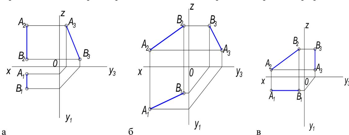
42. Natural size of a line in general position – this is the hypotenuse of a right-angled triangle, one of the legs of which is the projection of this line on the plane, the other leg.....
